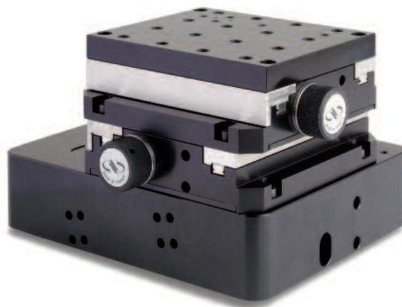
*Ultra low-profile precision XYZ system consisting of two VP-25XA linear stages and one VP-5ZA vertical translation stage. Compared to traditional stacks of stages, this solution offers a lower-profile alternative with easy access to the load from any side.*
