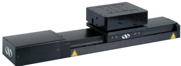
*A VP-5ZA stage mounted on top of an ILS linear stage (with optional VP-BP base plate). The vertical lift approach of the VP-5ZA allows centering of the payload over the bearings and close to the position feedback system. This avoids any cantilevered loads and results in more precise motion with higher load capacity.*
